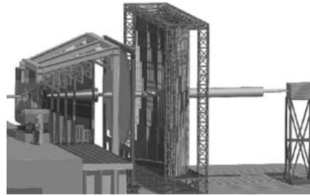
Fig. 5. CBM setup for muon measurements. The RICH detector of Fig. 4 is replaced by an absorber system interlayered with tracking devices.
