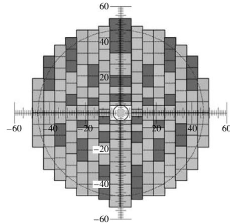
Fig. 6. Design of a STS station made up of double-sided silicon strip sensors.
