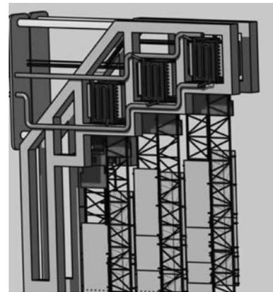
Fig. 7. Detail of STS system integration design, with mechanical support, front-end electronics and cooling.
