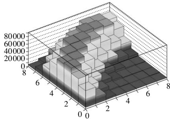
**Fig. 8.** Part of a Cherenkov ring observed in MAPMT tests with a proton beam in a plexiglass radiator.
