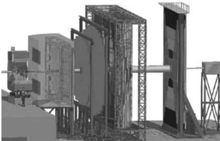
Fig. 4. CBM setup for electron and hadron measurements. The beam enters from the left. The vertex detector and the main tracking system are located inside the dipole magnet. Upstream are RICH and TRD for electron identification, TOF for hadron identification, the electromagnetic calorimeter and a forward calorimeter for event characterization.
