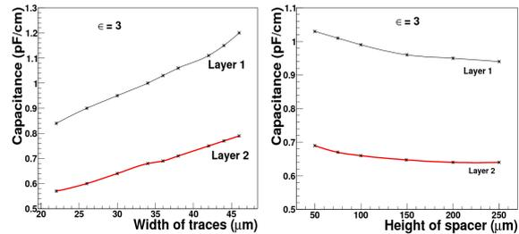
Figure 2: Line capacitance in the upper and lower signal layers as a function of the width of the traces (left) and the thickness of the spacer (right)
