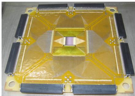
Figure 1: Demonstrator board 2b-4 with a CBM02 detector
