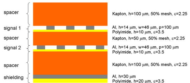
Figure 3: Cross section of the readout cable
