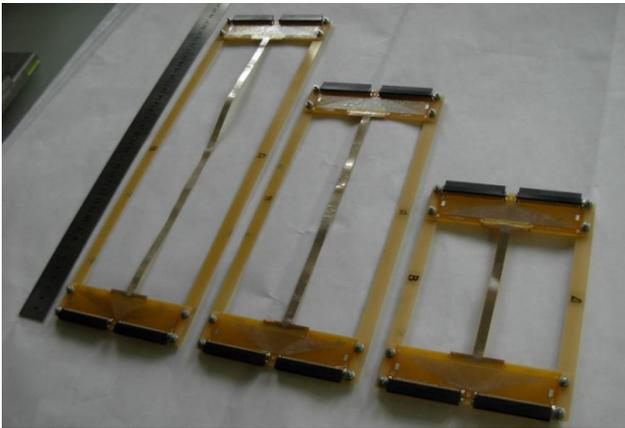
Figure 1: Different prototypes of microstrip line cables
