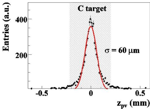
Figure 1: Z-distribution of the reconstructed primary vertex. The dashed region corresponds to the carbon target. The 3-prong vertex was considered as a  $D^+$  decay candidate if it was found more then  $450 \mu\text{m}$  ( $7.5\sigma$ ) downstream the target.
