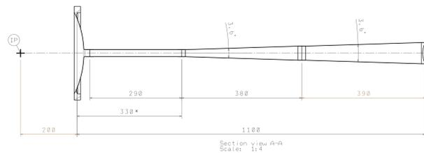
Figure 1: Tentative design of the STS beam pipe
