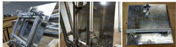
Figure 3: Mirror tiles mounting options. Left: base case (aluminum rectangle). middle: 3 independent mounts. Right: 2 aluminum bars.
