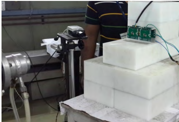
Figure 1: Neutron test setup at the VECC Cyclotron
