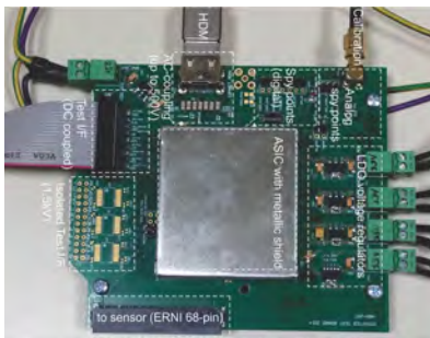
Figure 1: Test PCB for the STS-XYTER ASIC
