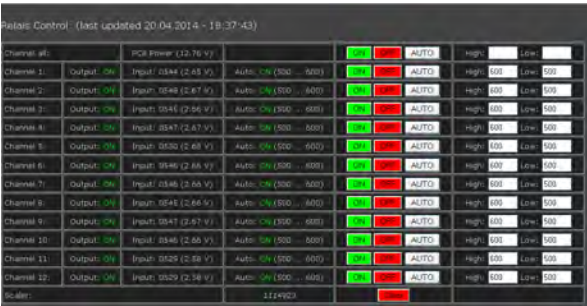
Figure 3: Control output of the monitoring system
