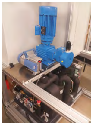
Figure 2: Vacuum pump set-up with condensing unit
