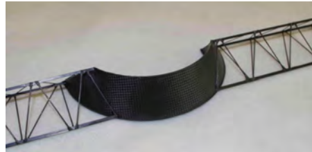
Figure 2: Prototype CF frame of a central ladder
