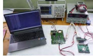
Figure 2: FEB under testing
