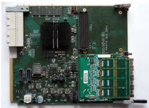
Figure 1: The AFCK board with an FMC card with 4 SFP+ cages connected to the FMC2 connector.
