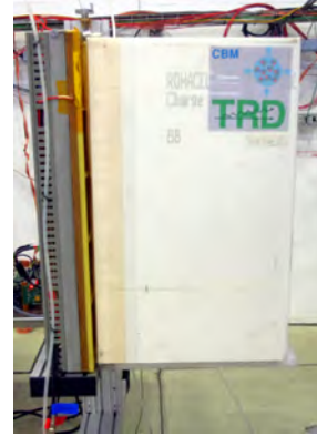
Figure 2: Side view of a real-size TRD prototype in the PS/T9 beam line in 2014 with a mounted full size foam foil radiator.
