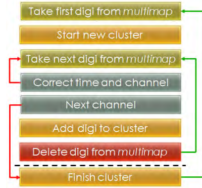
Figure 1: Simple scheme of the time-based clustering algorithm
