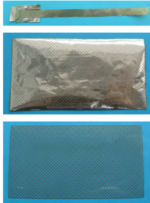
Figure 1: Analogue cable with narrow meshed spacer (top); shielding layer with wide meshed spacer (middle); wide meshed spacer (bottom).
