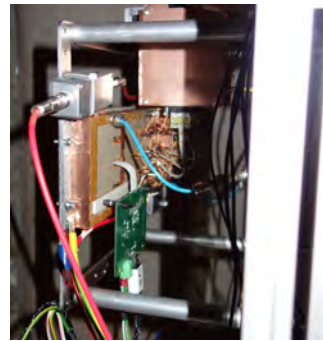
Figure 2: Side view on the setup used at CERN-SPS. The TRD prototype is rotated by 180° in comparison to Fig. 1 and also the SPADIC is mounted tilted by 90°, so that only the back side of the front-end board is visible.
