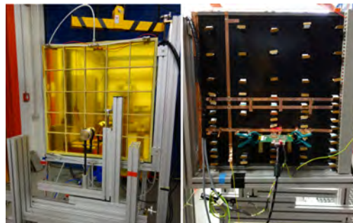
Figure 2: View onto both sides of the CBM-TRD detector prototype. In the left picture the position of the collimated ^{55}\text{Fe} can be recognized. In the right picture the chamber is shown from the front-end electronic side. One pad group of two rows with each 16 channels is read out with a single SPADICv1.0 [5].
